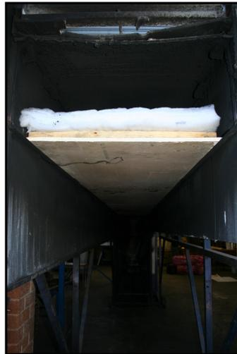
*Figure 3.1.2: Test installation above ceiling prior to ignition of fire source*
